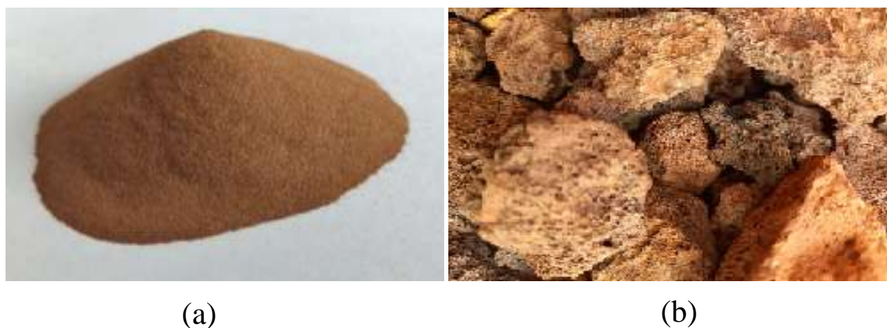
Fig. (4). Natural Jordanian Zeolitic tuff (a) as powder, (b) in nature.
