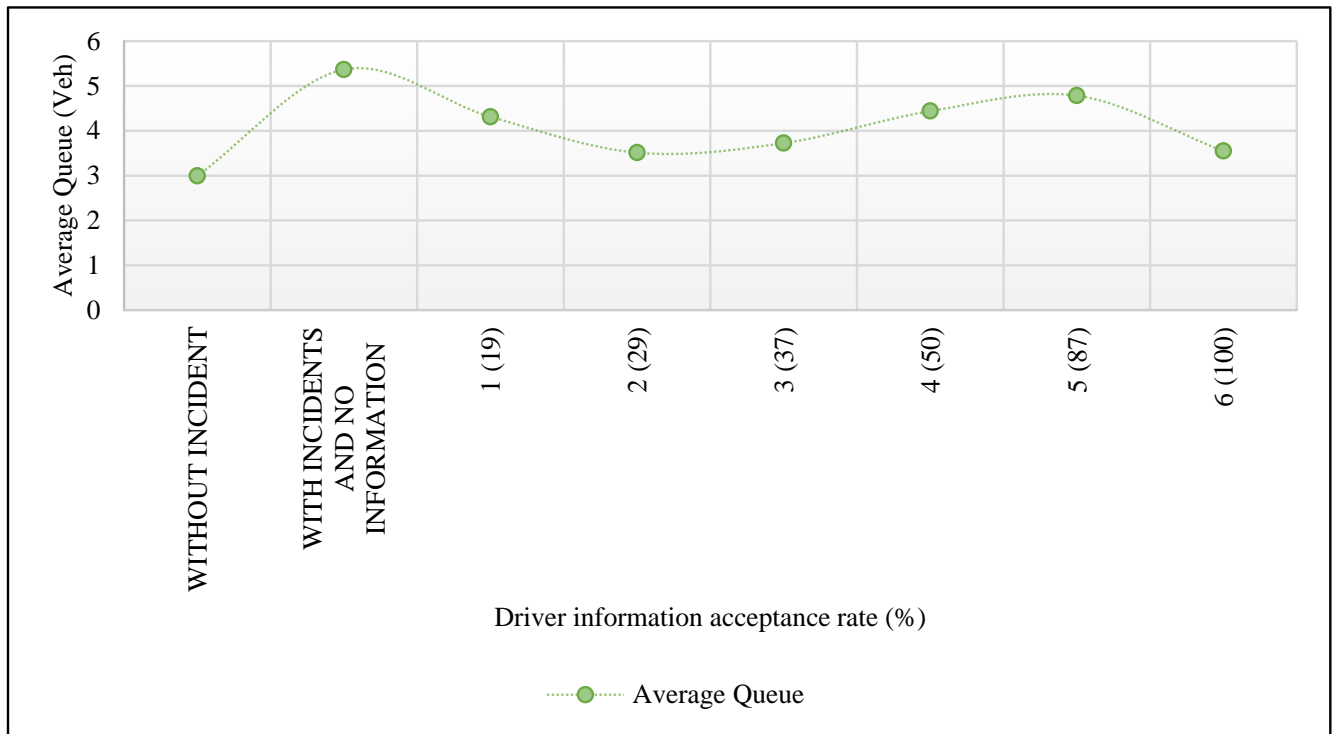
Fig. (24). Variation in average queue length across scenarios according to user information acceptance rates in the influence area of street 33 and street 48.
