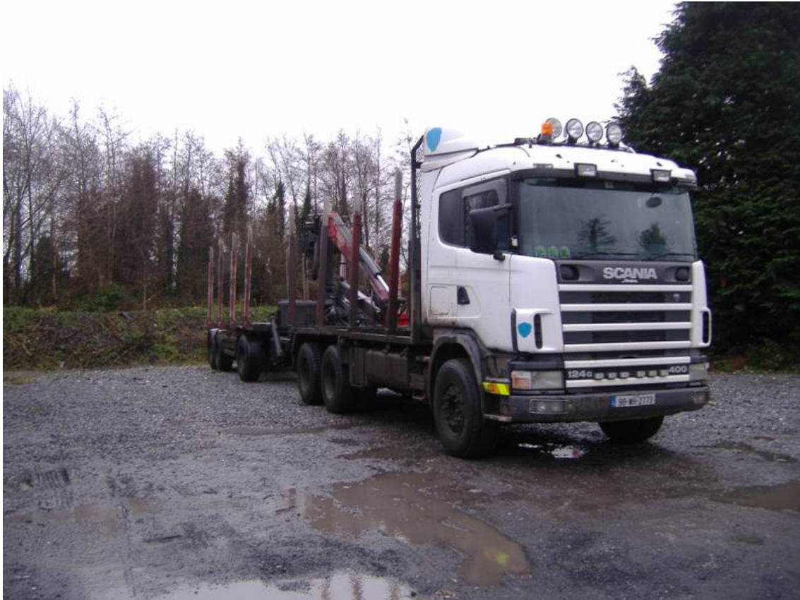
Fig. (4). Scania 124 (400) rigid + trailer + crane configuration.
